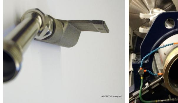
Optimized coolant conditions ID grinding
